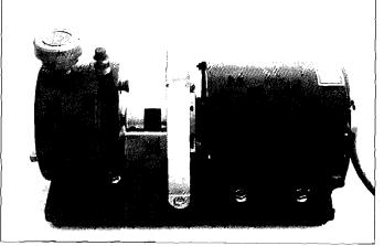
The rotary vane type pump is powered by an electric motor, is much more expensive to buy than venturi type pumps but is much more economical to operate
