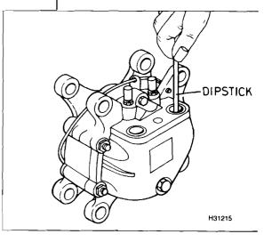
Using a dipstick to check the oil level on a York rotary vane compressor
