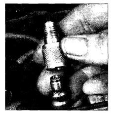
A typical high side adapter fitting like this must be used with the General Motors post-1976 type (3/8-24 thread) high side service valve before the hose can be attached
