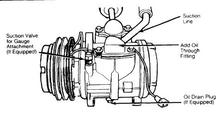
If the compressor on your vehicle has a drain plug, remove it and drain the oil, then reinstall the plug with a new O-ring - if it doesn't have a drain plug, you will have to remove the compressor, turn it upside down and drain the oil out of the suction and discharge ports
