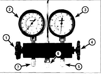
A typical manifold gauge set has . . .
