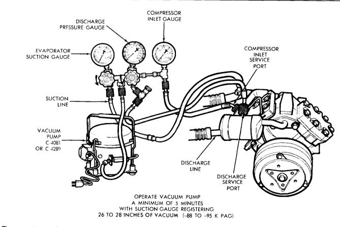
The correct setup for evacuating the typical non-accumulator system (Chrysler shown, others similar) - note that the center service hose of the manifold gauge set is attached to the inlet fitting of the vacuum pump
