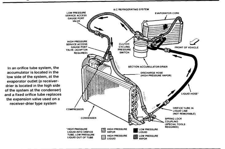
fice Tube (CCOT). Ford calls its system Ford Fixed Orifice Tube (FFOT). Earlier orifice tube systems used a standard thermostatic switch which turned the compressor off and on in accordance with evaporator temperature. Most newer systems have a pressure-sensing switch that controls compressor operation in accordance with system pressure. Measuring pressure is more accurate and responsive than measuring temperature.
