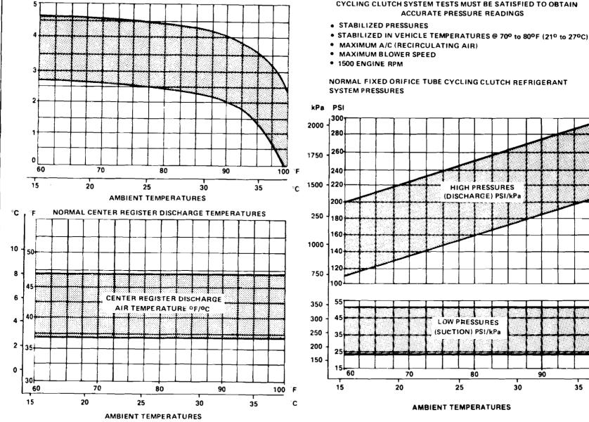
Refer to these charts to determine the normal clutch cycle rates and times and pressure/temperature relationships for Ford Fixed Orifice Tube (FFOT) system on F-100 through F-350 trucks and Broncos
