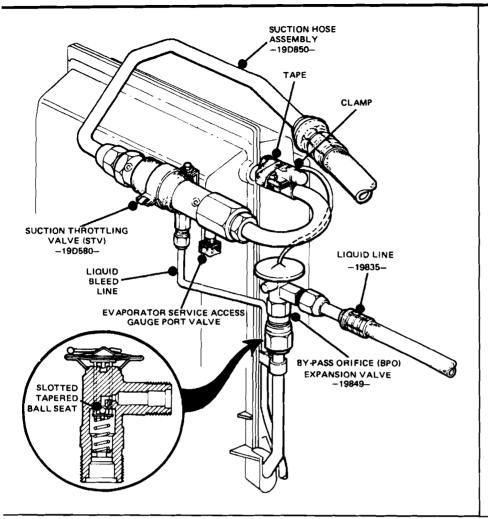
Ford Motor Company's By-pass Orifice (BPO) expansion valve uses a ball and slotted seat arrangementthe slotted seat keeps the valve from closing completely, allowing a small amount of refrigerant to flow into the evaporator, thus providing additional refrigerant and oil to the compressor for lubrication and cooling when the system is not operating at capacity - upper illustration shows location of principal components of assembly at evaporator, lower cutaway shows operation of the valve
