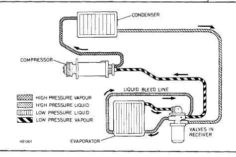
A typical Valves-In-Receiver (VIR) system
