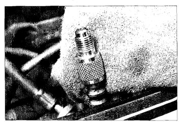
It's a good idea to protect the surrounding area of the engine compartment, and your eyes and skin, from refrigerant and oil with a shop rag when tightening or loosening a high side adapter fitting
