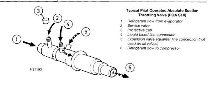
sure in the evaporator then increases, which raises the temperature and prevents icing on the outside of the evaporator. The opening and closing cycle of the valve continues as long as the compressor is running.
