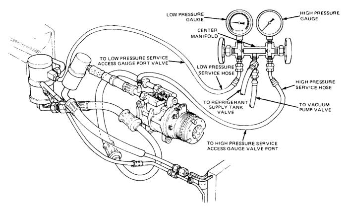
This is what the gauges look like when you start the vacuum pump: both gauges read zero - and the low side gauge will continue to drop below zero into the vacuum range as the pump sucks the system dry - the reading you're looking for is at least 25 in-Hg and even 30, if you can get it
