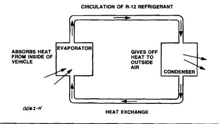
In its simplest terms, refrigerant absorbs heat from the passenger compartment at the evaporator, transfers it through a tube and sheds it to the outside air at the condenser ized by the compressor, the condensation point is raised above the temperature of the outside air. Thus, the heat transfers from the condensing refrigerant to the outside air. The fixed orifice tube and the compressor simply create pressure conditions that allow the third law of nature to work.
