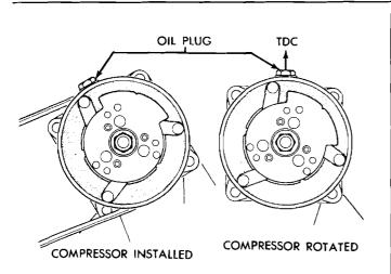
When you put the compressor on the workbench, make sure that the oil filler plug is at the top
