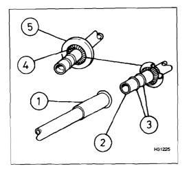
Spring-lock refrigerant line coupling components
