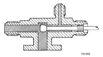
Stem-type service valve in mid (test) position
