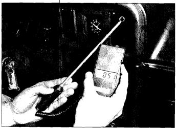
The best place to check the output of the evaporator is at the dash vent nearest the evaporator (usually one of the center vents)
