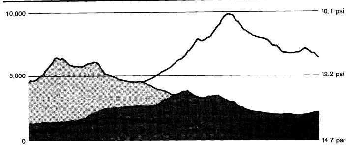
The higher the elevation, the lower the atmospheric pressure and the greater the necessary gauge correction)
