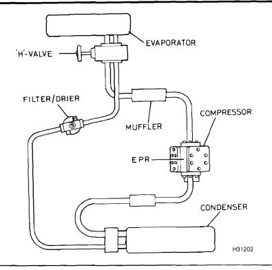
A typical Evaporator Pressure Regulator (EPR) system
