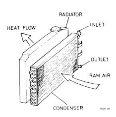
The condenser looks and works just like a heater core, evaporator or radiator and is always installed right in front of the radiator to receive the full airflow from the vehicle's forward motion
