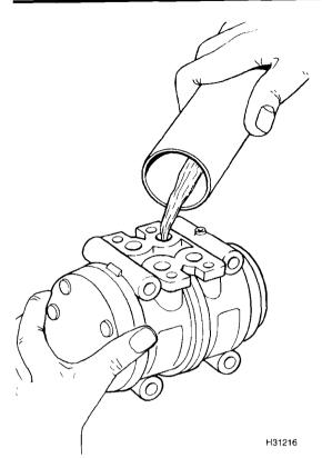
Refilling a Nippondenso 10-cylinder compressor with oil **9** Inspect the O-rings on the suction and discharge fittings and coat them with clean refrigerant oil before installing the lines.
