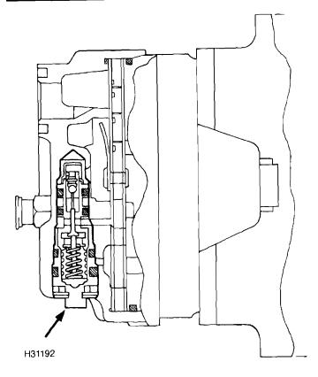
Cutaway view of rear of typical variable displacement compressor, showing crankcase pressure control valve location (arrow) switching the compressor off at a preset temperature and back on again at another preset temperature. Some switches are adjustable so that the compressor switching can be controlled in accordance with the requirements of the system and the vehicle occupants.
