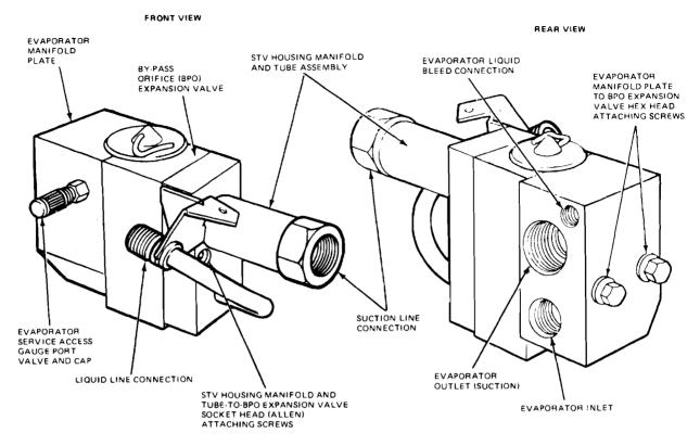
Ford Motor Company's By-pass Orifice (BPO) combination valve also uses the ball and slotted seat arrangement (upper illustration shows principal features of valve, lower cutaway shows operation of the valve)
