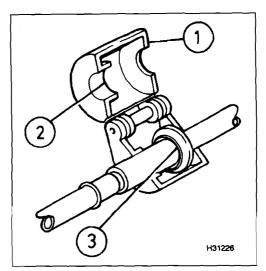
Fit the tool (1) over the spring-lock coupling with the projecting boss (2) against the open garter spring (3)
