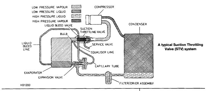
fer in configuration but, functionally, they're all pretty similar. Basically, all of them maintain proper evaporator temperatures by modulating evaporator pressure. The compressor in an STV system runs continuously instead of being cycled on and off. This type of system is no longer in favor with the manufacturers because it requires too much energy (fuel) for operation.
