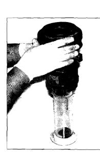
Carefully pour the lubricant in the compressor into a graduated container so that you can determine how much oil was in there
