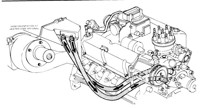
The easiest way to find the heater hoses is to locate them where they come out of the firewall, then trace them forward and detach them from the water pump and intake manifold (or block) - as a rule of thumb, you should force clean water through the heater hoses and the heater core in the direction opposite normal flow (the hose attached to the water pump carries coolant back to the engine, so that's the one you want to use)
