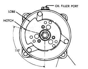
Rotate the hub plate lobe until the index notch is 110° from bottom dead center
