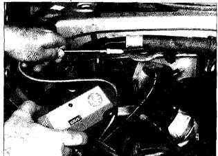
When using an electronic leak detector, search for leaks by slowly moving the sensing tip near all system components, controls, seals and fittings - the instrument will emit an audible alarm when the sensing tip detects the presence of refrigerant gases
