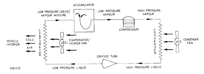
Basic air conditioning system using an orifice tube
