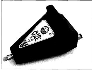
Venturi type vacuum pumps operate on compressed air (about 80 to 90 psi air power from a compressor) to pull down a vacuum in the system in about 1/2hour - this type of pump is inexpensive to buy, but uses a lot of electricity (to run the compressor for 1/2-hour)
