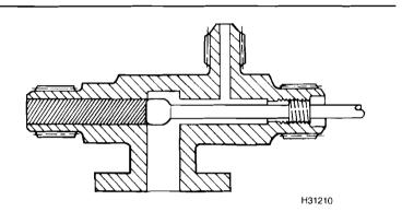
Stem-type service valve in front-seated (closed) position
