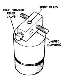
The receiver-drier performs two functions: it acts as a storage tank for the liquid refrigerant until it's required by the evaporator and it protects the system by absorbing moisture from the R-12 into a "desiccant bag" of silica gel
