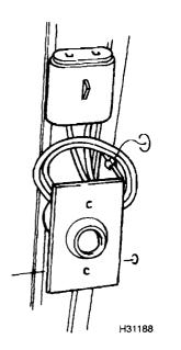
Typical ambient temperature switch, located at front of vehicle, behind grille panel
