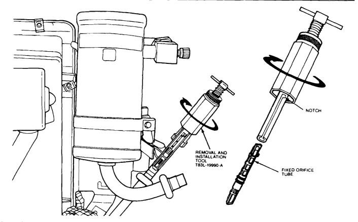
Insert the special tool into the tube, turn the tool clockwise to engage the tangs on the tube, then turn tool nut slowly to avoid breaking the orifice tube during removal
