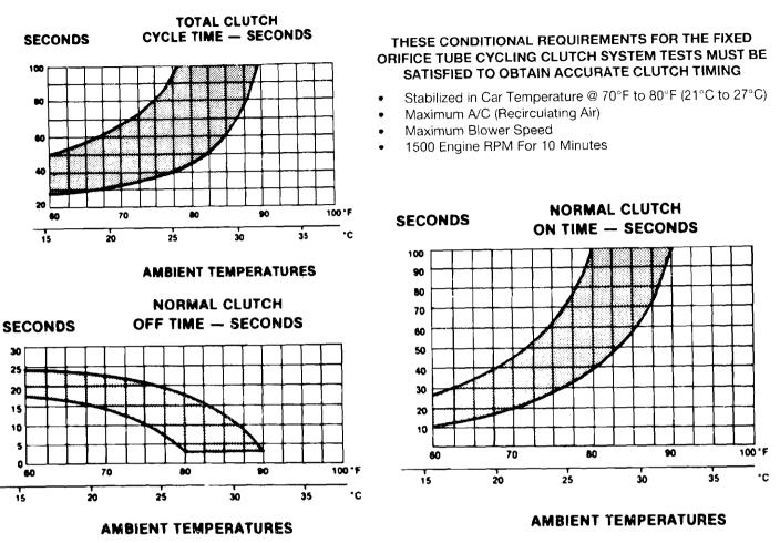
Refer to these charts to determine the normal clutch cycle rates and times for a Ford Fixed Orifice Tube (FFOT) system -Tempo/Topaz, Escort/Lynx shown - others similar
