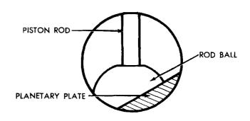
To verify that the hub plate lobe and index notch are aligned, look through the oil fill hole and verify that the ball end of the top piston rod lines up with the fill hole
