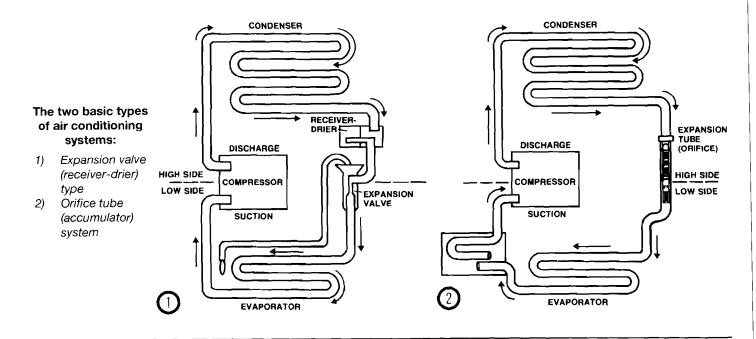
The compressor raises the pressure (and the temperature) so the refrigerant can condense and release heat as it moves through the condenser. A "pressure differential" is created at the expansion valve or orifice tube - the dividing point on the front side of the system. We will explain the expansion valve and orifice tube in detail later in this chapter.
