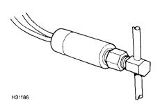
Typical high pressure cut-out switch, located in refrigerant line
