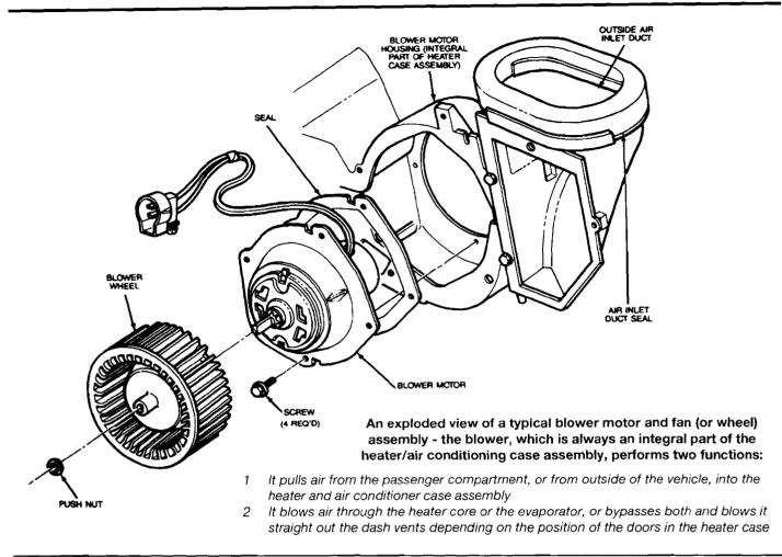
core), also located in the evaporator housing. The blower (see illustration) draws warm air from the passenger compartment over the evaporator and blows the "cooled" air out into the passenger area. The blower motor is controlled by a fan switch with settings from Low to High.
